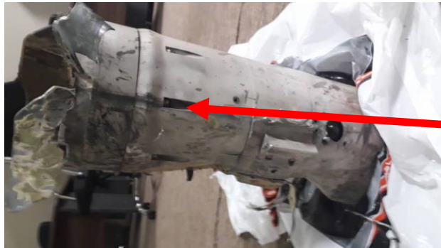
A. Imagery of missile remnant Note: Reduction in fuselage diameter (identifiable after “trumpeting” due to impact)
