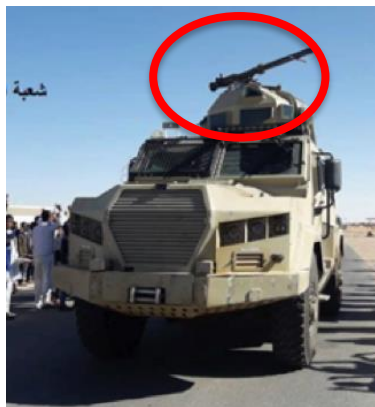
Figure B.36.3 KADDB Al Wahsh PPV modified with an 73mm SPG-9 recoilless gun fitted to 'snakehead' cupola c
