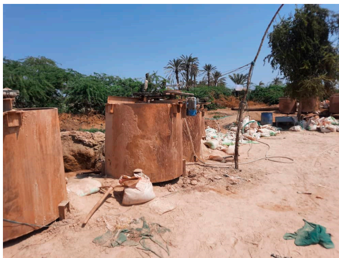
Figure A1. Tank agitators used in the study area. Source: authors' data. Photo taken in January 2023.
